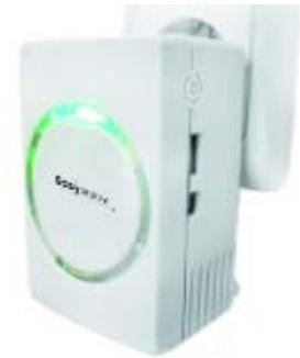
The **Easywave CCserv** server comes fully configured. If settings are changed at a later date, they can be adapted to your needs using a web browser. In order to do this, it is necessary to connect the **Easywave CCserv** to a PC/notebook via LAN or WLAN.
