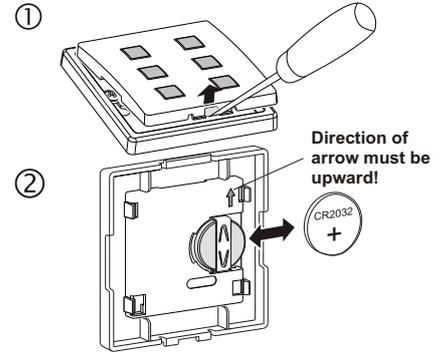
**Note:** The transmitter's coding is preserved even if there is no voltage supply. You do not need to re-register the code with the wireless control after a battery change.
