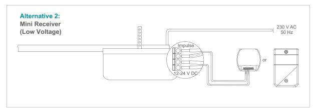
Provide Mini Receiver with the power supply of the garage door, connect the control line to the garage door and then adapt the hand transmitter.
