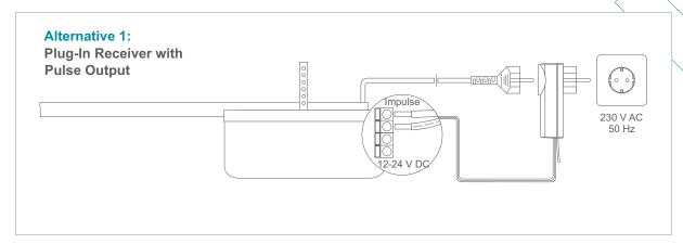
Just insert Plug-In Receiver into the power socket, connect control line to the garage door and then adapt the hand transmitter.
