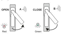
OFF/ON (RTS26E5001A03): If the window is opened, the Easywave code B (OFF) is sent and if the window is closed the Easywave code A (ON) is sent
